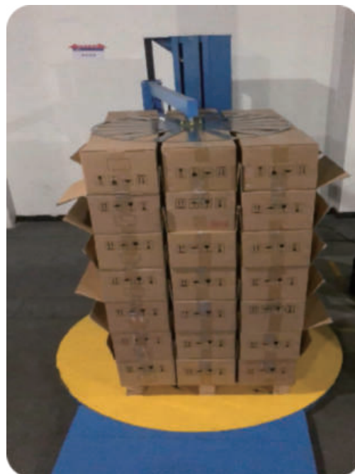
Automatic Film Winding Machine Replacing Manual Winding
